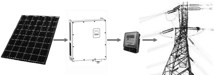
Figure 1: Application of Photovoltaic Grid-Connected Inverter in Photovoltaic Generating System.
